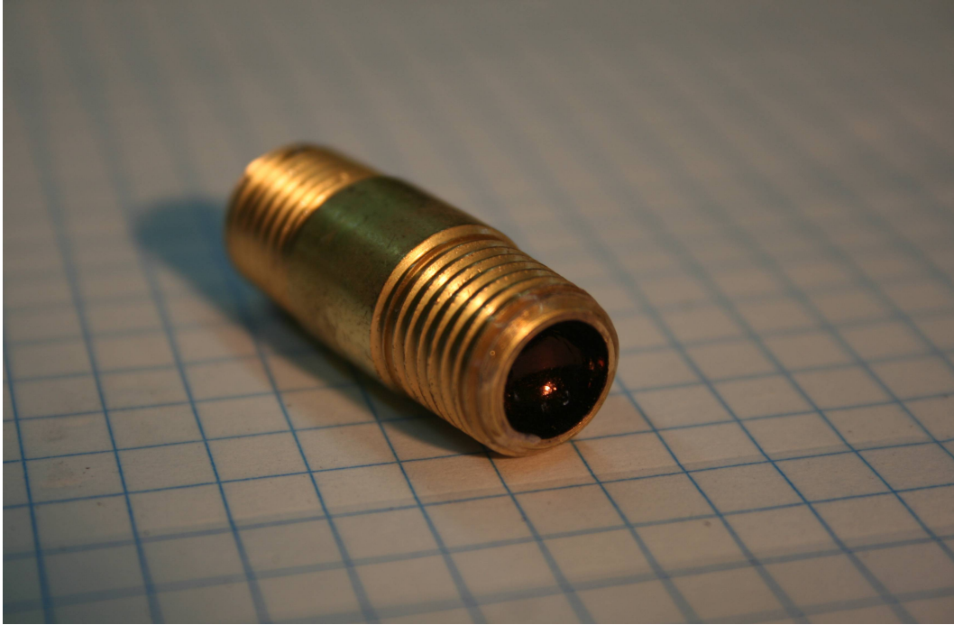
Add-on Vacuum System -- Blocked Mounting Fitting
